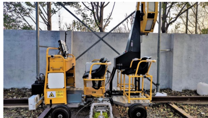
Intelligent integrated track inspection vehicle
