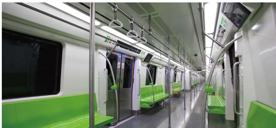
Upgraded the lighting system on Line 14 trains to LED lights
