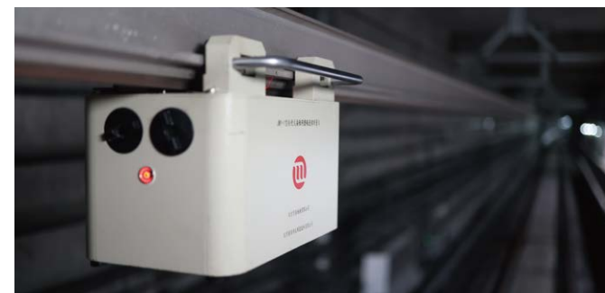
Portable Continuous Wear Measurement Device for Contact Wires
